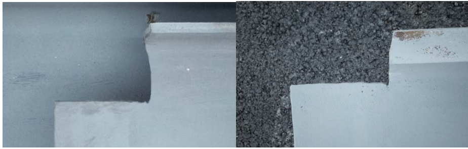
Figure 6. Poor beam cope cutting practices
