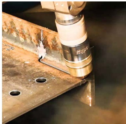
Figure 7. Controlled beam cope cut
