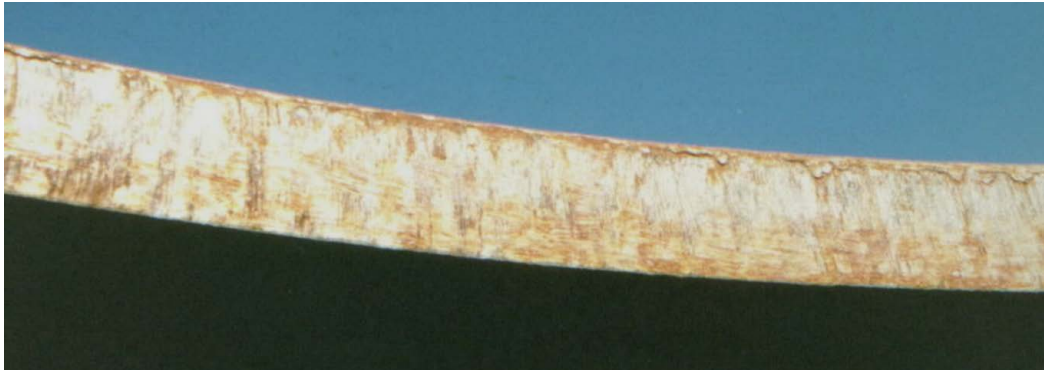
Figure 12. Example of an RBS cut edge
