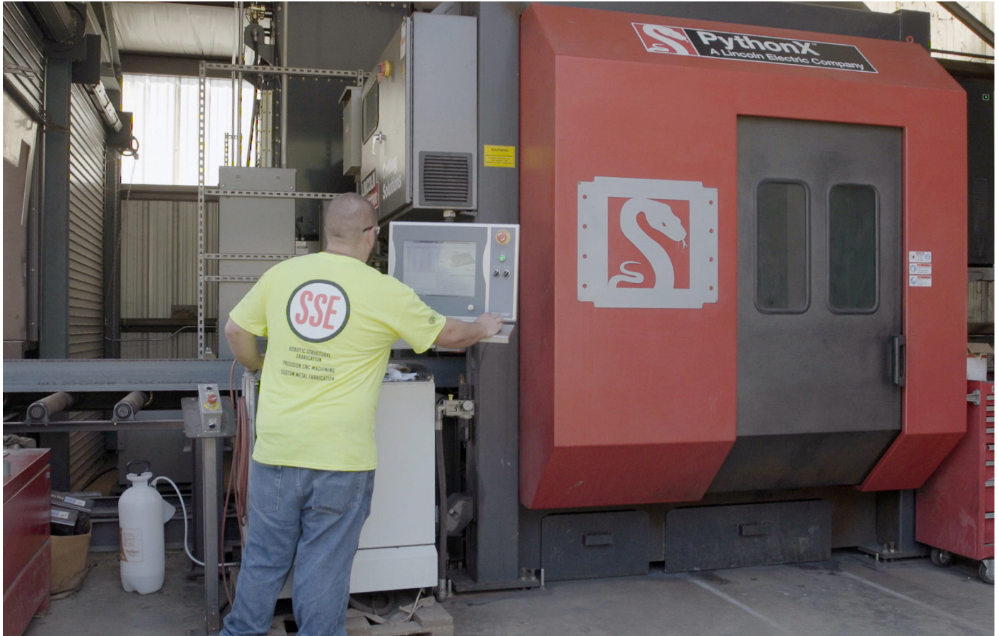
Operator programming the PythonX for beam production
