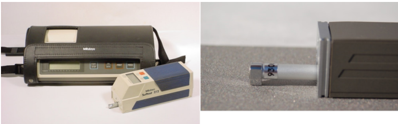
Figure 26. Contact-type surface roughness instrument
