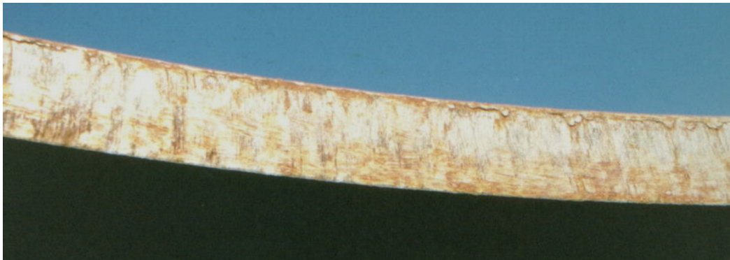
Figure 12. Example of an RBS cut edge
