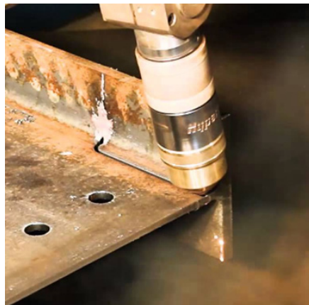
Figure 7. Controlled beam cope cut
