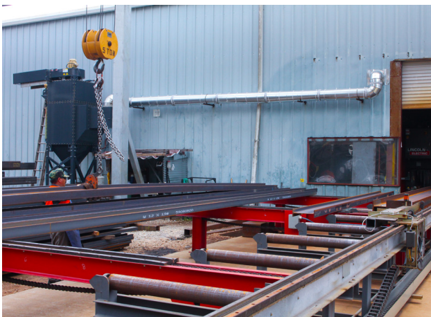
Cross Transfers and Infeed Conveyor were installed outside of the building due to space restrictions
