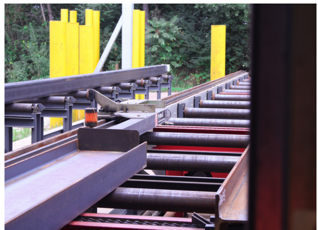
Cross Transfers and Infeed Conveyor were installed outside of the building due to space restrictions
