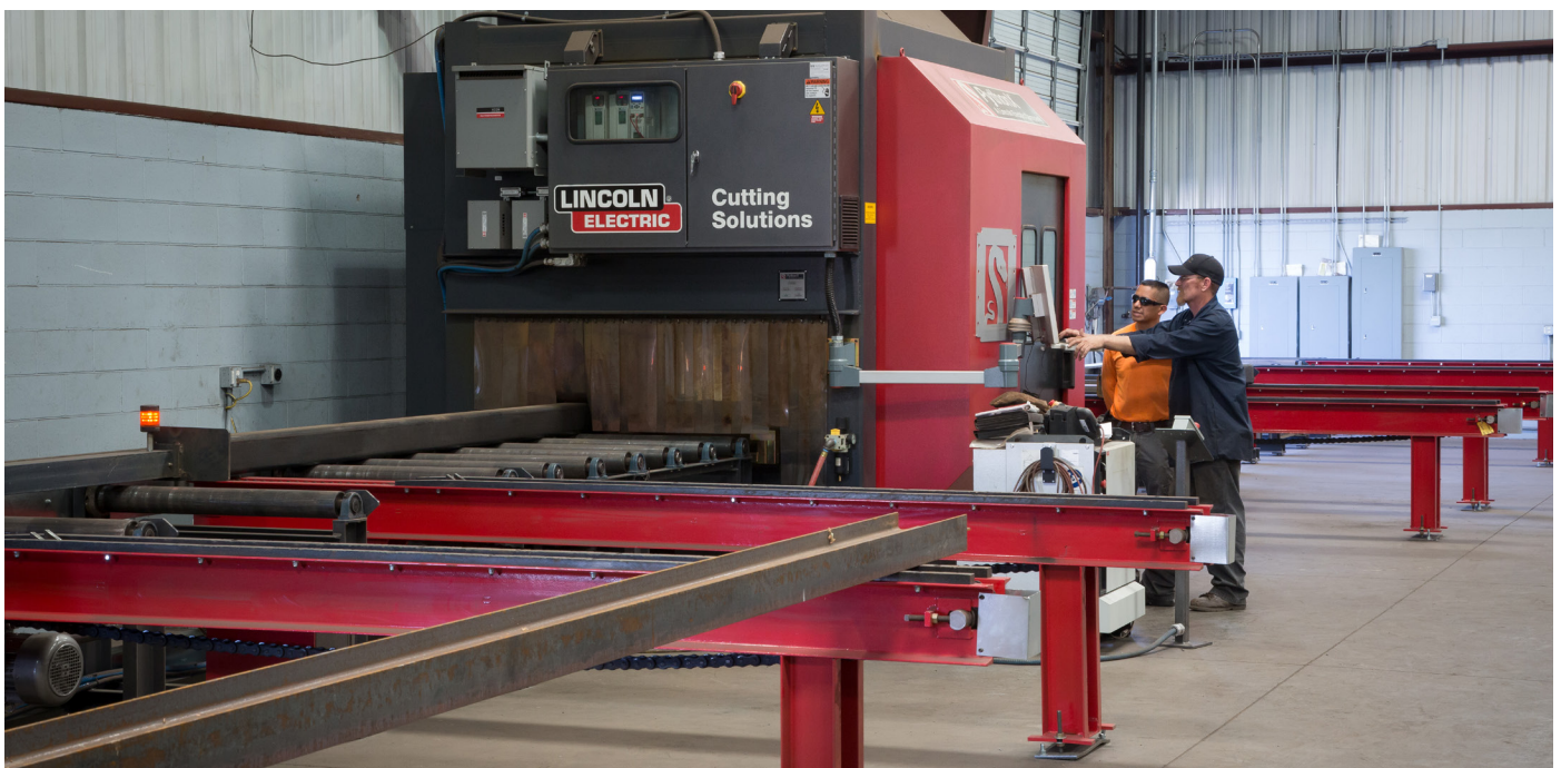
Operator programming the PythonX for beam production
