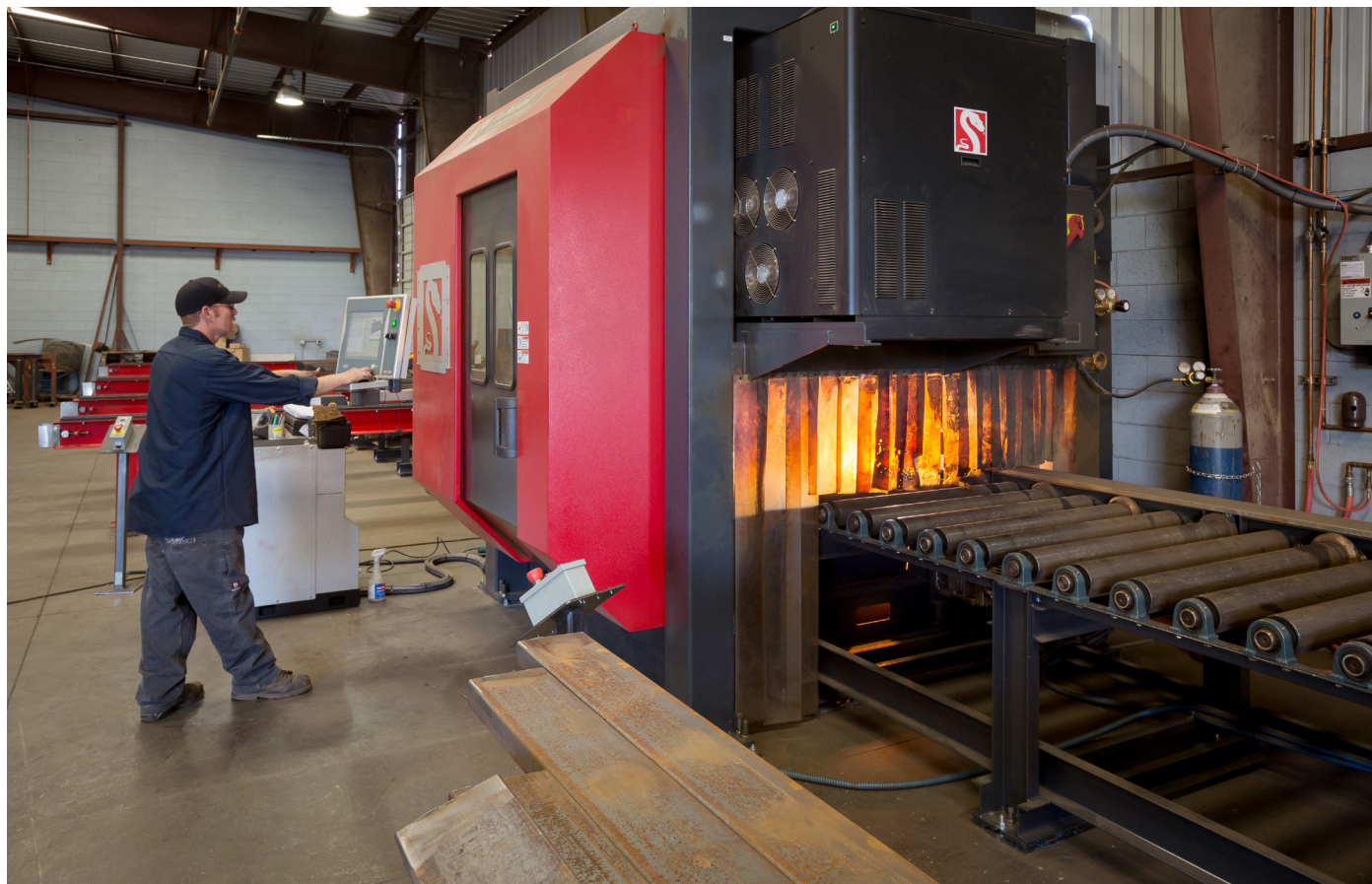
PythonX processing a structural steel beam
